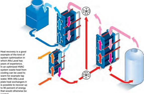
Heat recovery is a good example of the kind of system optimization in which Alfa Laval has years of experience. In an optimized HVAC cooling can be used to warm for example tap water. With Alfa Laval to 95 percent of energy that would otherwise be wasted.
